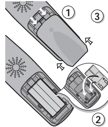
1. Remove the battery cover by pressing on the indent and sliding downward.
