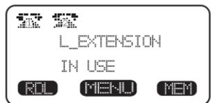
When one or both lines are currently in use by a parallel set (a telephone device other than your GIGAPHONE system, all registered Handsets and Base will display:
