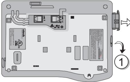
1. Open the spare battery charger by pressing the release button, located on the left-hand side of the Base Unit. A drawer will open to reveal the spare battery compartment.
