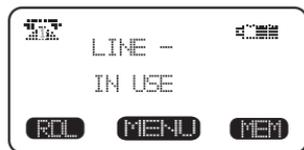
When both lines are in use at the same time, the **L\_EXTENSION IN USE** message will alternate between 1 and 2.
