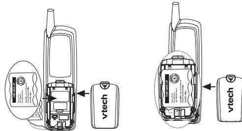
3. Align the cover flat against the battery compartment, then slide it upwards until it clicks into place.
