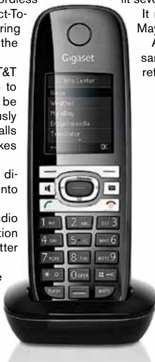
Gigaset's C610A IP DECT phone is a hybrid landline/VOiP model.
