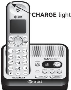
4. Charge the handset by placing it face up in the telephone base. The **CHARGE** light is on when charging.
