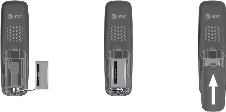
1. Plug the battery connector securely into the socket inside the handset battery compartment, matching the color-coded label.
