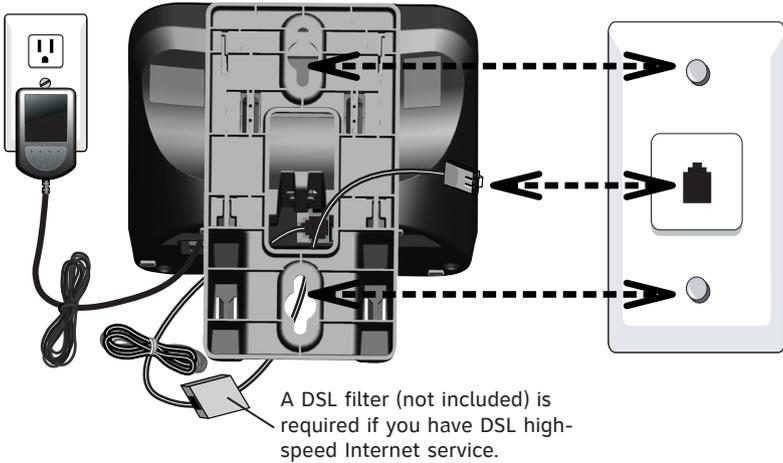
5. Align the holes on the wall mount bracket with the mounting studs of the wall mounting plate and slide the bracket down until it locks securely. Bundle the telephone line cord and power adapter cord neatly with twist ties.
