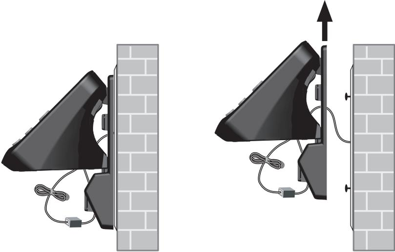
3. Lift the telephone base up to detach it from the wall mount bracket.
